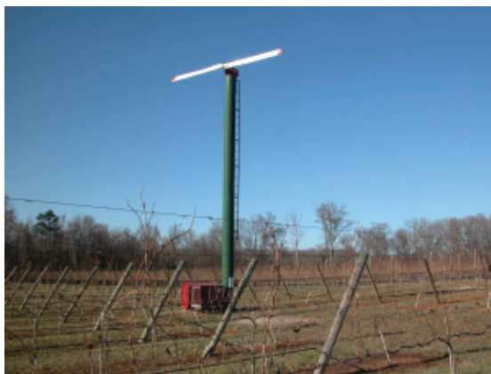
Figure 4.4. This Orchard-Rite wind machine stands 35 feet above the vineyard floor and has a 125 HP gas-powered engine that turns the 19-foot fan. It protects a 7-acre vineyard in Davidson County. (Photo taken by Barclay Poling, December 18, 2005)
